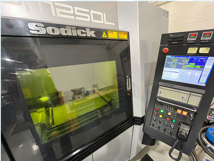
SODICK OPM250L combines industry-leading laser sintering technology with high-speed milling to print and finish a product in one automated operation.
